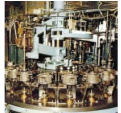
The moulds of the automatic glass-making machine have to be changed and cleaned every 24 hours
