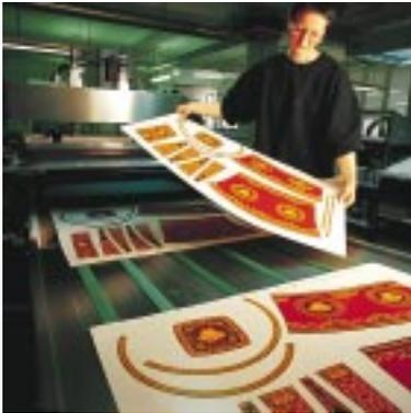
Checking of the transfer sheets after the final print
