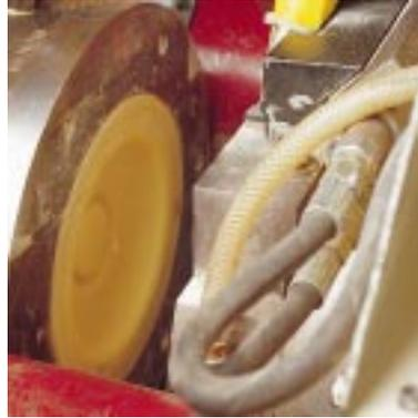
Open mould of isostatic plate press
