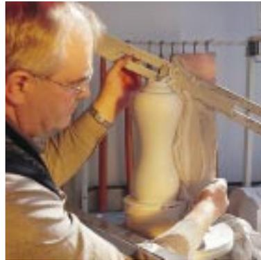
The model of a vase is turned from a plaster cylinder
