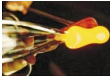
The glassblower attaches a small knob of molten glass to the bottom of the bowl...
