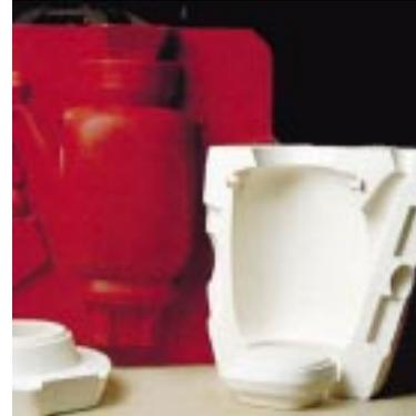
On the left the synthetic resin mould, on the right the negative casting mould
