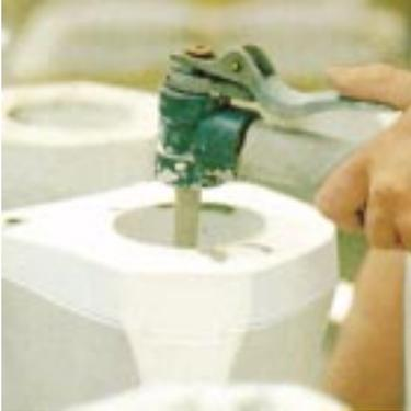
Pouring the slip into a mould made of plaster-of-paris
