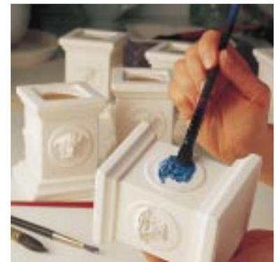
The relief is being coated with a blue wax to prevent it from being glazed.
