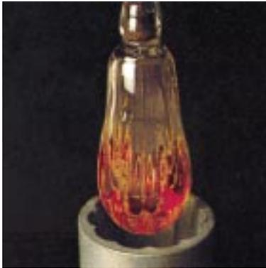
A relief is imprinted by blowing the glass into a primary mould
