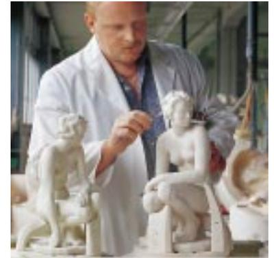
Special supports are needed during firing to prevent the porcelain from becoming distorted
