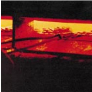
Knives are hardened by heating and then chilled with cold air.
