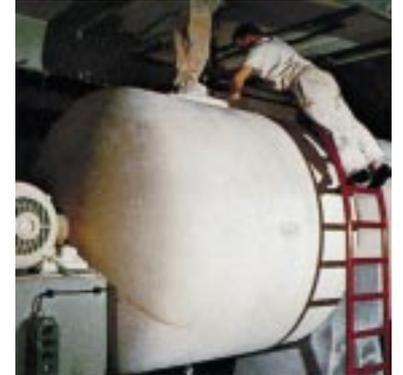
The raw materials are loaded into the drum mill
