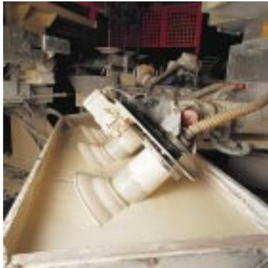
A machine dips the plates into a bath of glaze turning them at the same time
