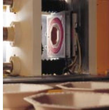
Open mould used in press casting
