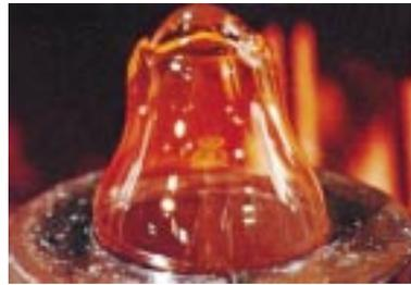
The bowl of the glass is turned continuously as it is blown in to a metal mould
