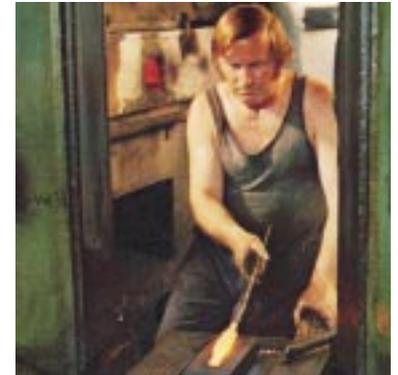
The forging hammer is dropped on to the red-hot knife with a force of 70 tons
