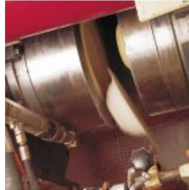
An elastic conveyor belt catches the plate made from porcelain granules
