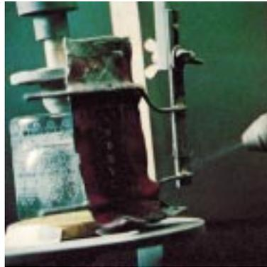
A decoration is given a matt finish with a sandblasting gun using a rubber stencil
