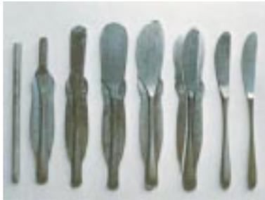
The various stages of shaping a knife from a single metal rod
